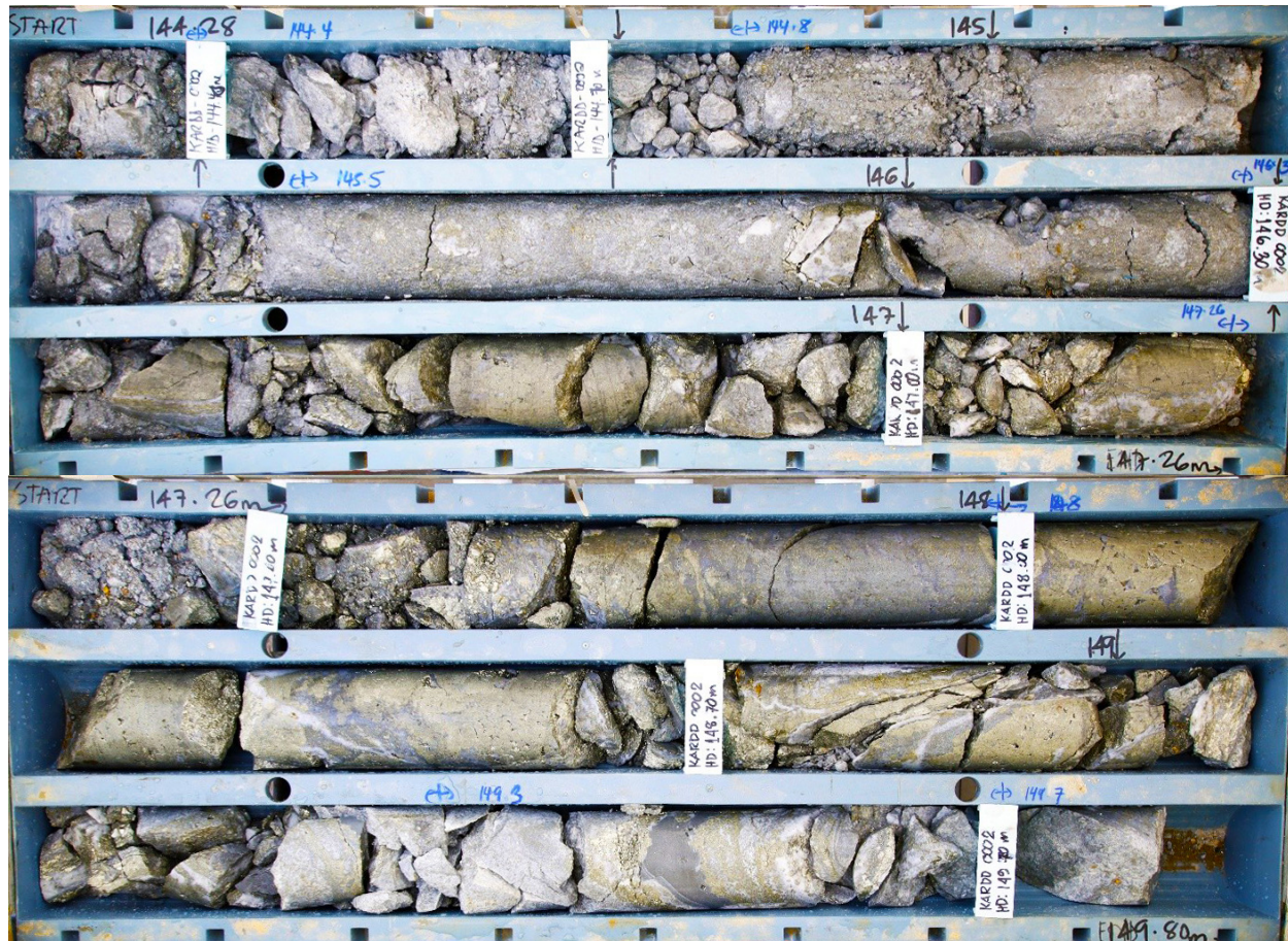
KARDD002, 144.28 – 149.80m; within intersection of 7.2m at 24.44 g/t Au, 0.10 % Cu, 13 g/t Ag.
